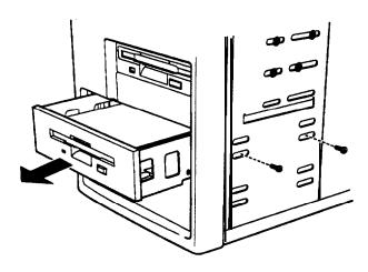
3. If you are not installing an externally accessible drive in the open drive bay, you need to install a drive slot cover for that bay. Push the slot cover into the open bay until the tabs on the cover click into place.
